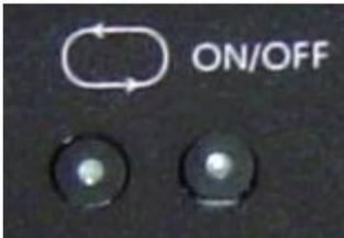
**To activate Hardware control:** Hold the On/Off Button for 5 seconds until you hear one beep which activates the H/W Control function. The LED lights in the front panel should continuously flash and you can hear the relay clicking when activated.
